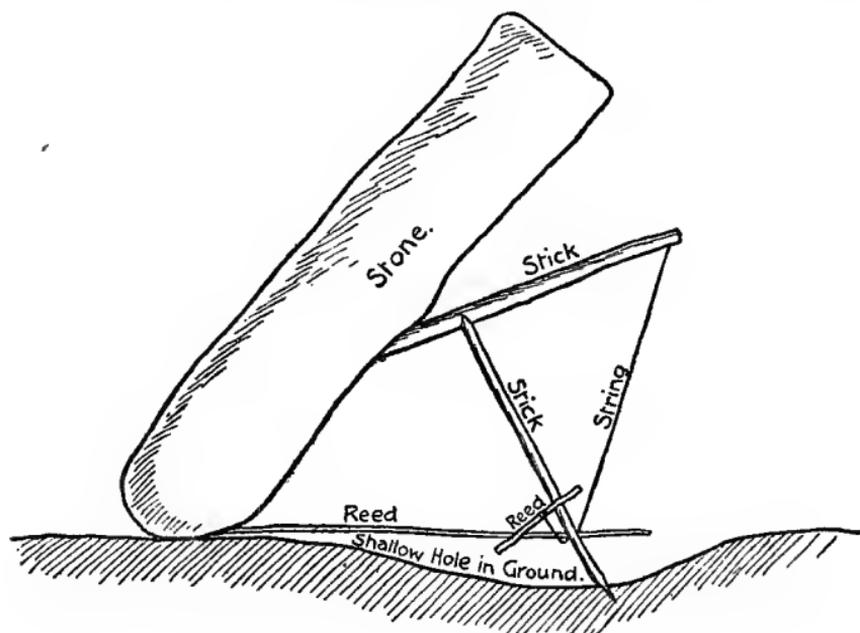
so that no bird may be able to get at it without touching the trigger of the trap, which instantly releases the stone, so that it crushes the bird. Another very common form of trap is made with a number of pieces of reed which are stuck in the earth so that they form an inverted cone. A small opening is left at one side of the cone, and in this opening a hair from
